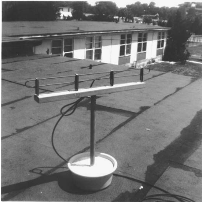
136 MHz dipole - part of the crossed baseline interferometer
