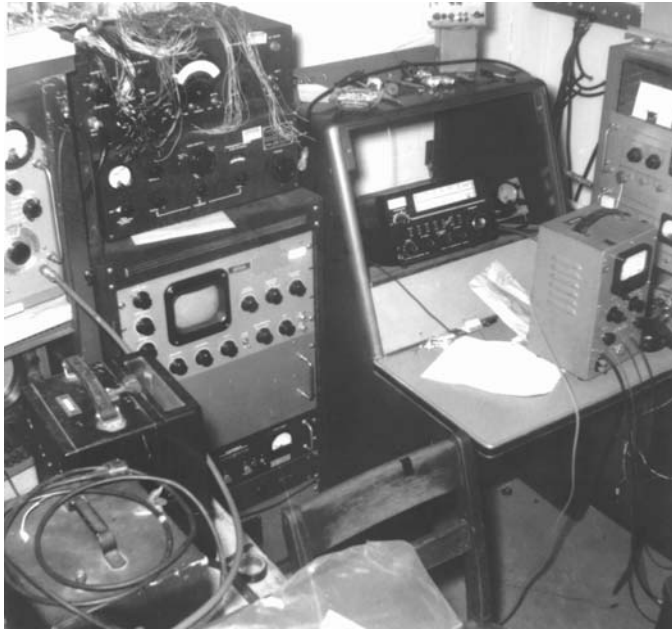
Tracking console - Drake IIB receiver in center, HP608 on left
